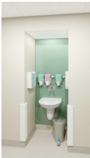
Figure 2.9: Reduced height ceiling within a corridor bay
